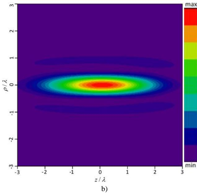
Fig.3. Calculated distributions of the intensity of the longitudinal component of the field of the  $TM_{01}$  mode with moderate (a) and sharp (b) focusing.
